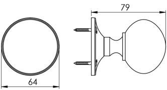
This unsprung mortice knob is suitable for use with most U.K. heavy duty tubular latches. For a new interior door installation we would recommend using our York heavy duty tubular latch from the list below.
