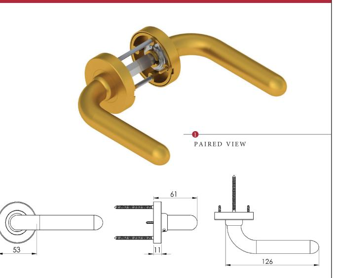
This latch handle is suitable for use with most U.K. tubular latches. For a new door installation we would recommend using our York standard tubular latch from the list below.
