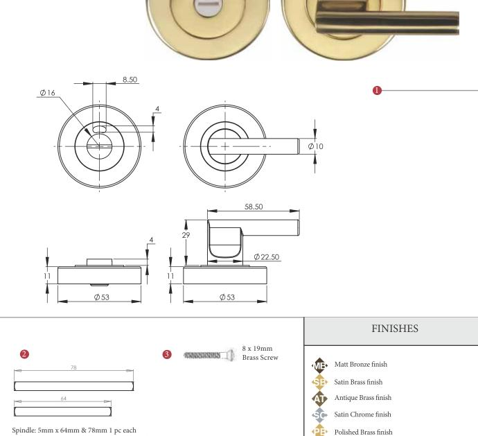
Spindle: 5mm x 64mm & 78mm 1 pc each 64mm spindle suitable for 35 & 45mm door thickness & 78mm spindle suitable for 54mm door thickness.
