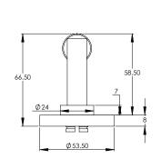
This latch handle is suitable for use with most U.K. tubular latches.
