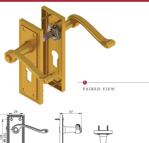
This lock handle is suitable for use with most U.K. Euro Profile cylinders and sashlocks with a 48mm CTC.
