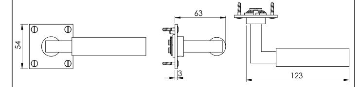
This latch handle is suitable for use with most U.K. tubular latches. For a new door installation we would recommend using our York standard tubular latch from the list below.
