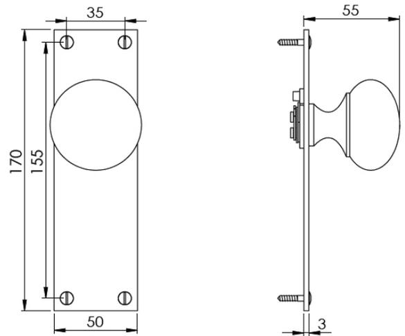
This mortice knob is suitable for use with most U.K. tubular latches.
