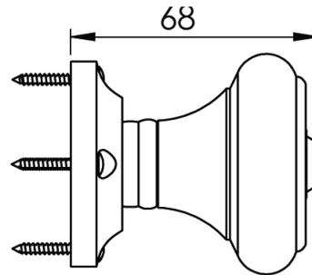
This mortice knob is suitable for use with most U.K. tubular latches.
