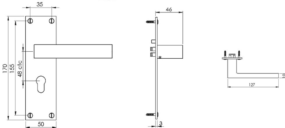
This lock handle is suitable for use with most U.K. Euro Profile cylinders and sashlocks with a 48mm CTC.
