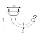
This lock handle is suitable for use with most U.K. Euro Profile cylinders and sashlocks with a 48mm CTC. For a new exterior door installation we would recommend for use with our York Euro Profile sashlock ref: YKCSLE29.CE (2.5") or YKCSLE39.CE (3"). A separate Euro Profile cylinder in a size to suit the door thickness will also be required to operate the lock mechanism.
