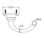
This lock handle is suitable for use with most U.K. Euro Profile cylinders and sashlocks with a 48mm CTC. For a new exterior door installation we would recommend for use with our York Euro Profile sashlock ref: YKCSLE29.CE (2.5") or YKCSLE39.CE (3"). A separate Euro Profile cylinder in a size to suit the door thickness will also be required to operate the lock mechanism.
