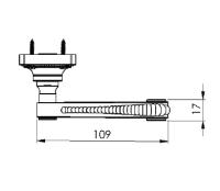
This lock handle is suitable for use with most U.K. Euro Profile cylinders and sashlocks with a 48mm CTC.
