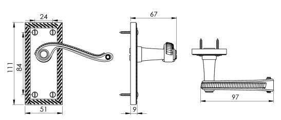
This latch handle is suitable for use with most U.K. tubular latches. For a new door installation we would recommend using our York standard tubular latch from the list below.
