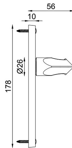
This latch handle is suitable for use with most U.K. tubular latches.
