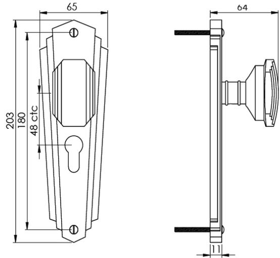
This lock handle is suitable for use with most U.K. Euro Profile cylinders and sashlocks with a 48mm CTC.
