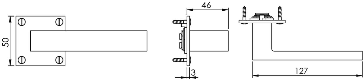
This latch handle is suitable for use with most U.K. tubular latches.
